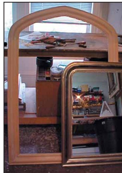
Photo 4: The blanks were joined in their respective positions, and the profile was carved so that the contours met neatly.
