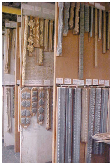
Just a few of the original models in the inventory of Abe Munn Picture Frames used in their multiple-head spindle carving machines.
